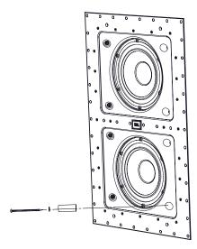
Now tighten the isolator mount screws. This assembly will expand the isolator mount to hold the subwoofer in the wall. The screws should be firmly tightened enough to expand the isolator mounts, but do not need to be tightened beyond this point.
