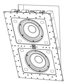
When the SSW-4 is in the wall, tighten the attachment screws at the top and bottom. This will bind the wall to the dogleg clamps at the ends of the subwoofer. DO NOT OVER-TIGHTEN – at this point, they only need to be firm.
