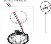
Use a screw driver to secure frame in the wall
