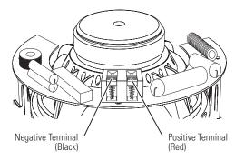
Press down on the terminal tab to open the hole; insert the bare end of the wire into the hole; and release the tab to secure the wire. NOTE: C383XC and C363XC models have post-type terminals. Press down on the post to open the hole; insert the bare end of the wire into the hole and release the post to secure the wire.
